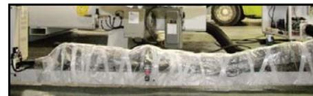
**STEP 3:** Attach all servo cables and wires. Use wire ties to secure in place. Connect and secure the Limit Switch wire on the X,Y, and Z-axes and attach the X,Y, and Z servo ground wires (if applicable).
