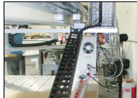
**STEP 4:** (Proceed to **STEP 6** if Microdrop Coolant System was not ordered) Connect the 3/8" airline to the Microdrop Coolant Unit. Make sure there are no kinks anywhere in the line. Secure with wire ties. (PICTURE 12)
